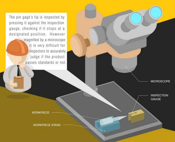
The pin gage is pressed against an inspection gauge with the tip stopping at its designated position. A pin gage with a large tip angle will not reach the designated position, while one with a small angle will exceed it (limit).
