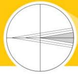
The standard tip angle of the pin gage is engraved on the built-in ocular micrometer in three reference lines so inspectors can immediately decide whether it passes inspection standards or not.
