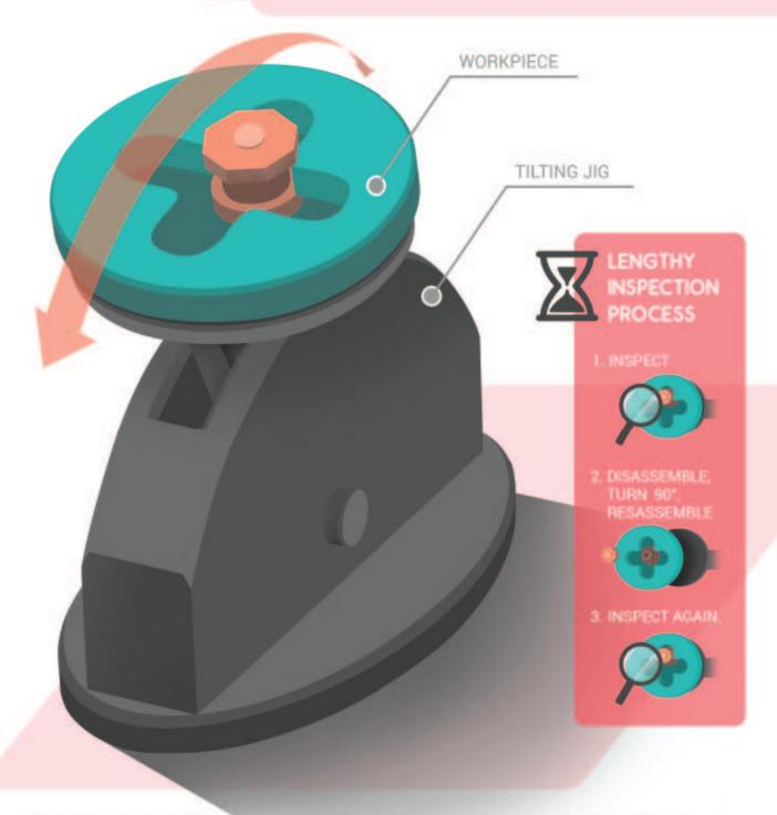
SINCE THE CURRENT TILTING JIG CAN ONLY BE MOVED IN TWO DIRECTIONS (FRONT AND BACK), ALL MOVEMENT ON THE WORKPIECE COULD NOT BE CHECKED IN ONE LOADING, SIGNIFICANTLY AFFECTING THE AMOUNT OF TIME WORKERS SPEND DURING INSPECTION.
